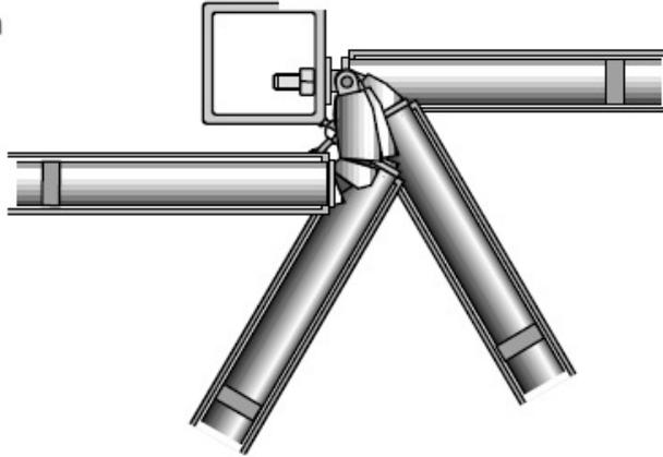
The LOCK-TEC RTS Tube Gate Closer is inserted into the door and connected to the counter plate (which is fixed to the frame) by an elastic joint with integrated steel ropes. When the gate is opened, the joint is pulled out and the closing spring is tensioned. The closing speed is controlled by the hydraulic damping cylinder in the middle of the closer. This closing speed is adjustable and therefore can be adapted to suit different requirements.
